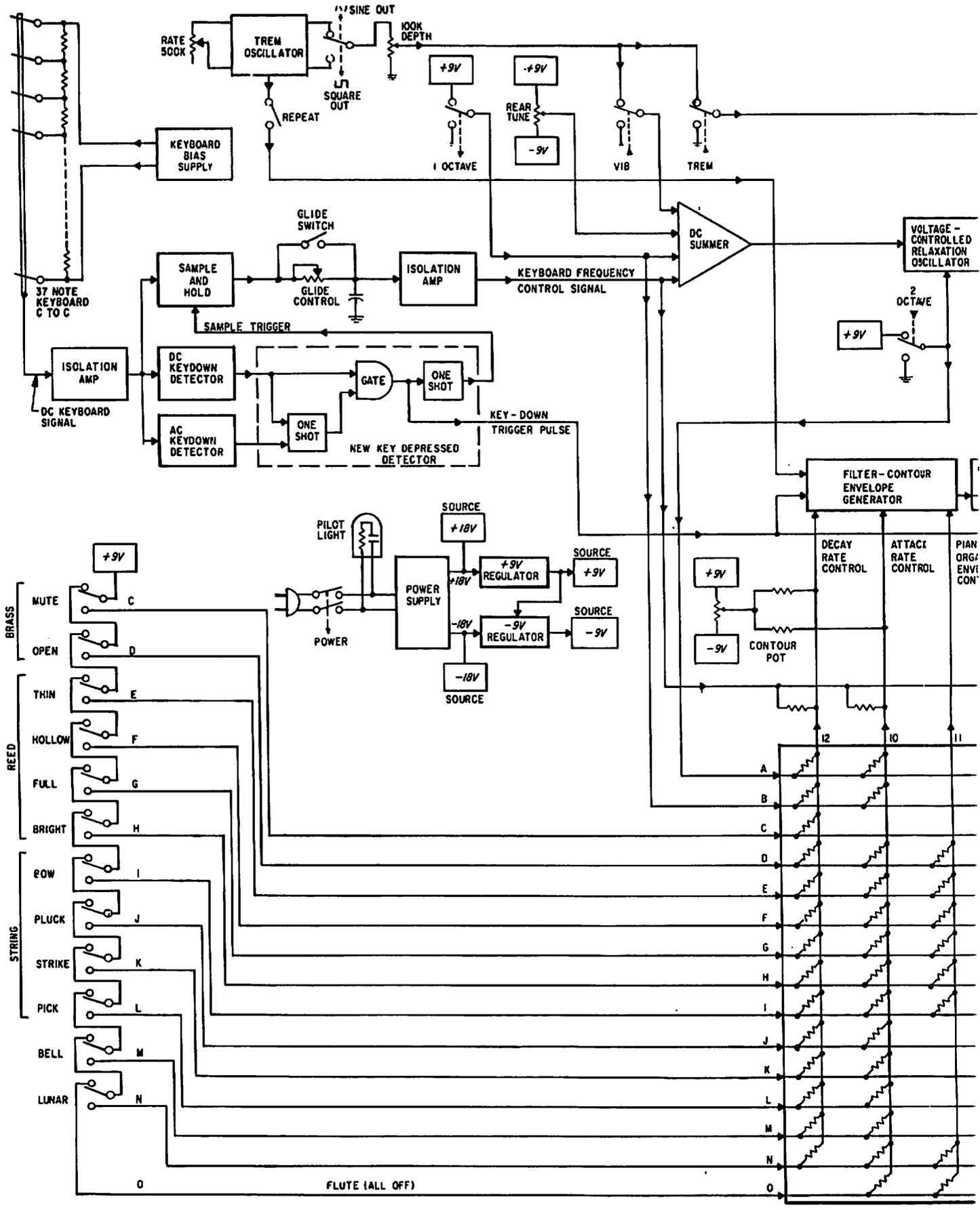
FIGURE 10-8 SATELLITE BLOCK DIAGRAM
