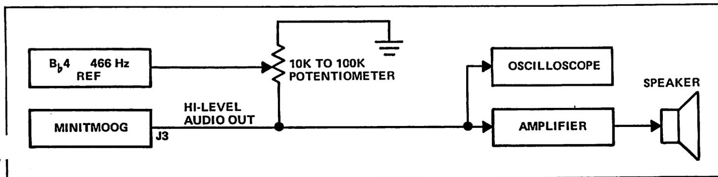
FIGURE 4-1 MINIMAL TEST SETUP FOR TUNING
