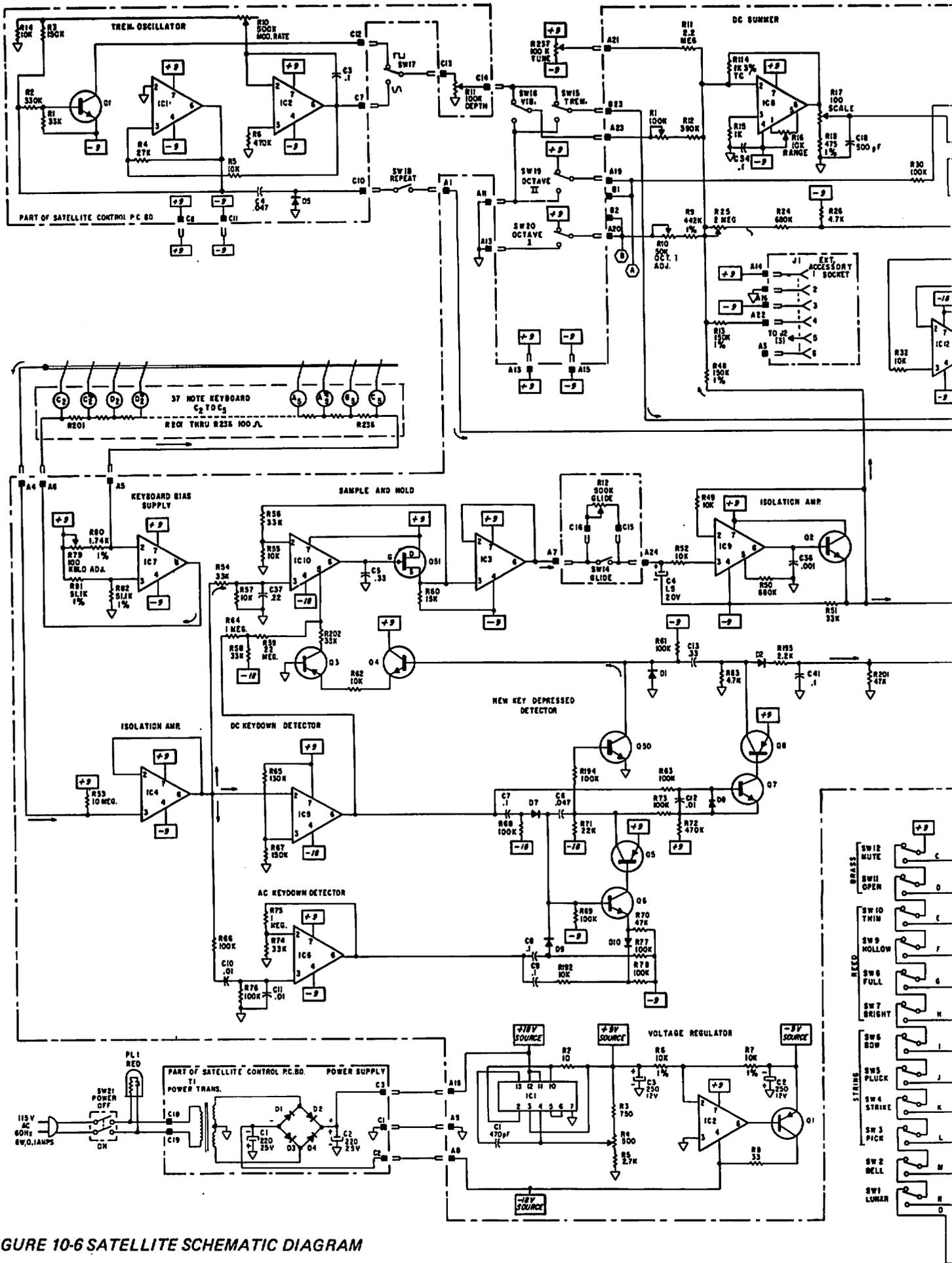
FIGURE 10-6 SATELLITE SCHEMATIC DIAGRAM
