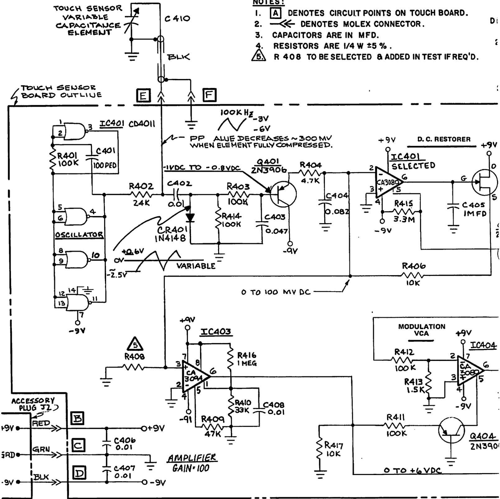
FIGURE 10-4 MINITMOOG TOUCH SENSOR BOARD ASSEMBY NO. 4 SCHEMATIC DIAGRAM
