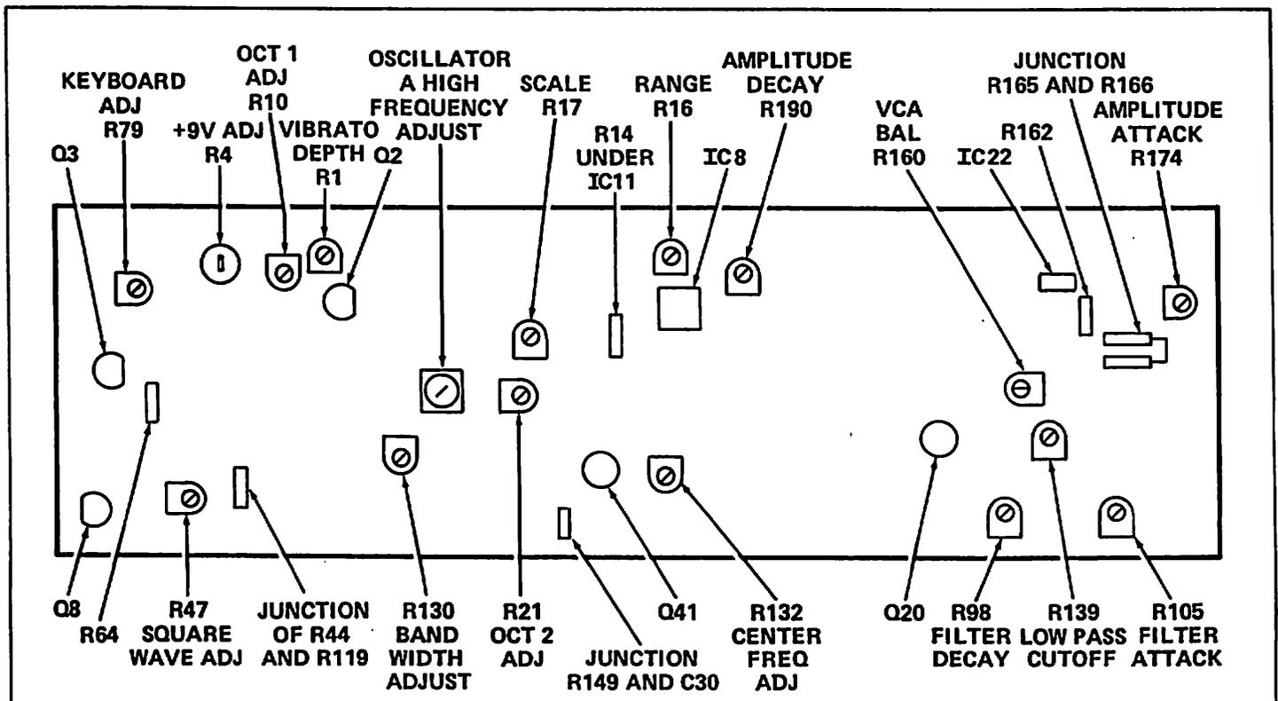
FIGURE 4-3 MAIN BOARD NO. 1 ADJUSTMENT CONTROLS AND OSCILLOSCOPE TEST POINT LOCATIONS
