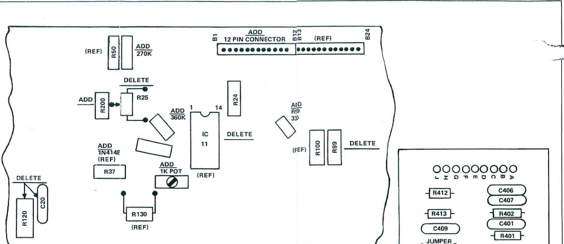
MODIFICATION OF SATELLITE PRINTED CIRCUIT BOARD TO CONFORM TO MINITMOOG CONFIGURATION
