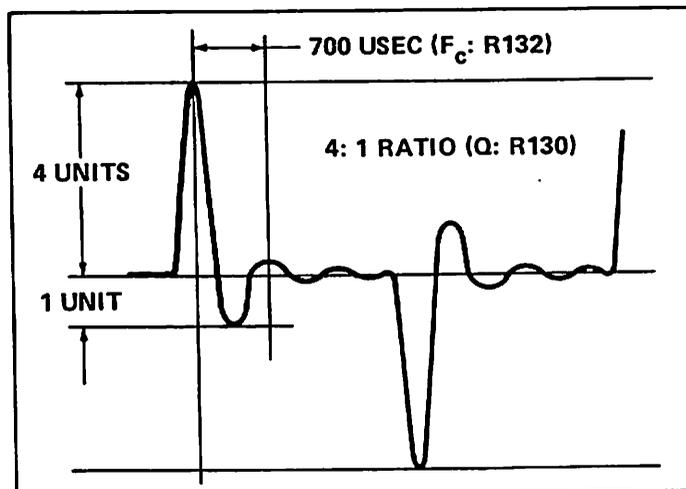
FIGURE 4-7 BAND PASS FILTER Q AND  $F_c$  AT Q41 SOURCE
