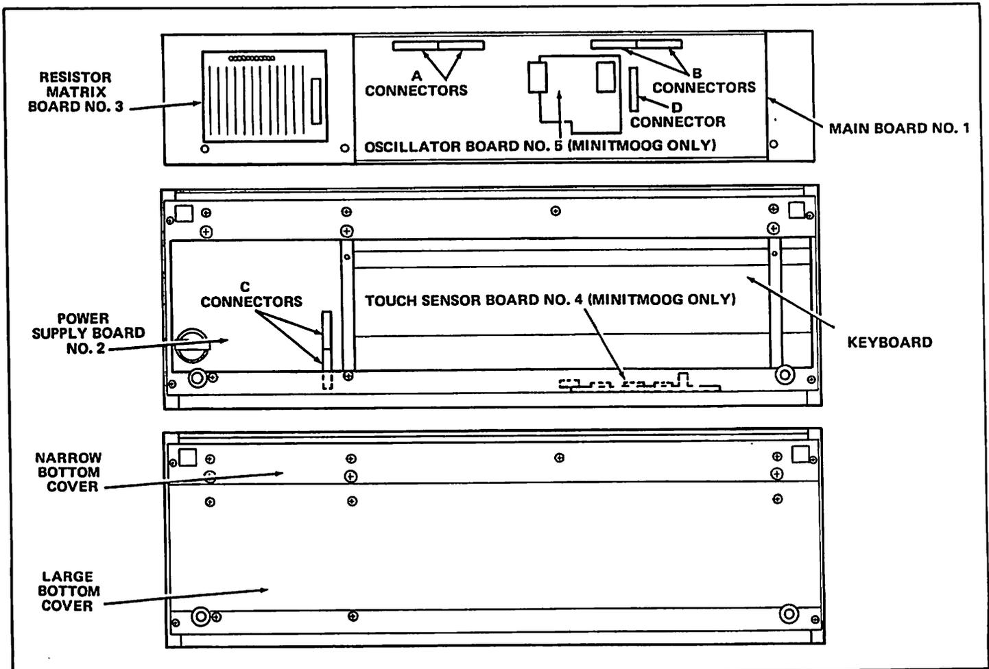
FIGURE 3-2 MINITMOOG COVER AND PRINTED CIRCUIT BOARD LOCATIONS (BOTTOM VIEWS)
