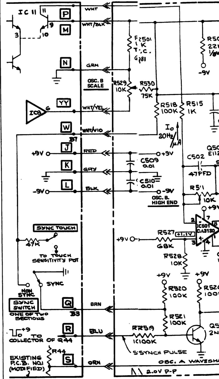
FIGURE 10-4 MINIMOOG TOUCH SENSOR BOARD ASSEMBLY NO. 4 SCHEMATIC DIAGRAM
