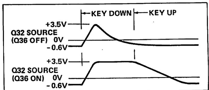
FIGURE 2-5 SOURCE VOLTAGE OF Q32
