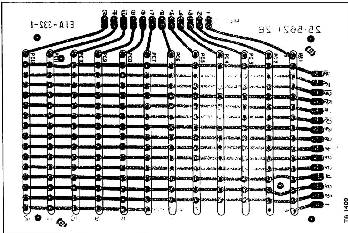
RESISTOR MATRIX PRINTED CIRCUIT BOARD ASSEMBLY
