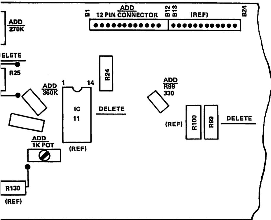
MODIFICATION OF SATELLITE PRINTED BOARD TO CONFORM TO MINITMOOG CONFIGURATION
