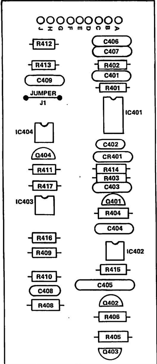
TOUCH SENSOR PRINTED CIRCUIT BOARD
