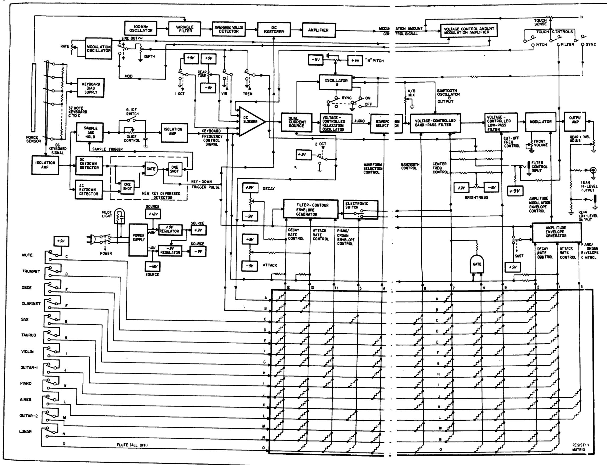
FIGURE 10-2 MINITMOOG BLOCK DIAGRAM
