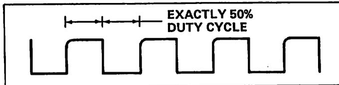
FIGURE 4-6 SQUARE WAVE AT JUNCTION OF R44 AND R119
