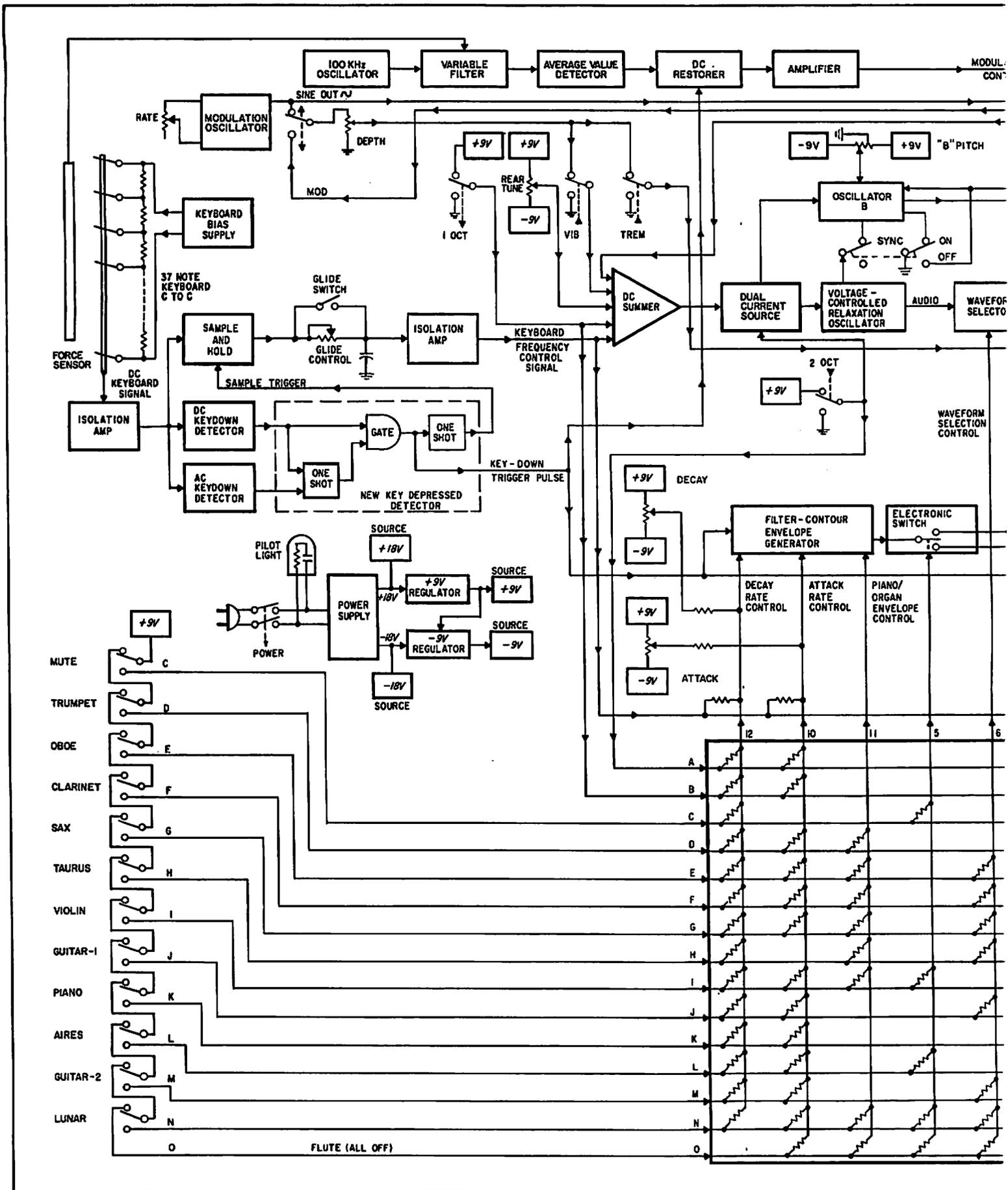
FIGURE 10-2 MINIMOOG BLOCK DIAGRAM
